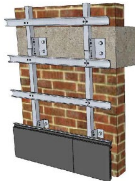
4. Hanging the panels on G-Channel
