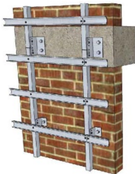
3. Installation and plumb of the horizontal profile on the vertical profile
