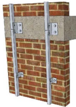
2. Level installation of the vertical profiles and plumb installation of the brackets
