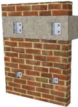
1. Layout and bracket installation
