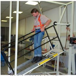
Netz tiles being tested at the factory in Germany
